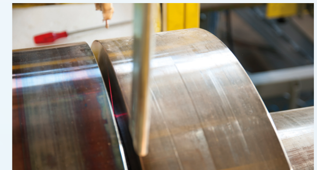
Narrow gap 17 mm - Laser scan mock up
