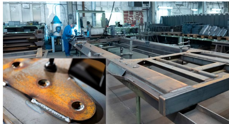
The innovative forceArc puls welding process is used in every area of steel construction for welding untreated black steel. Process reliability is high, and the virtually spatter-free seam is perfect.
