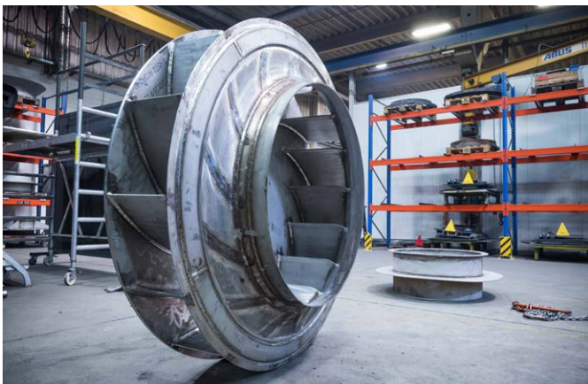
A welded fan wheel with a diameter of 3.5 metres. Including the reinforcement rings there are over 60 metres of weld seams in the component here.
