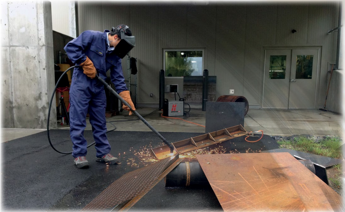
Plasma cutting torch, manual, extra-long torch neck, cutting and gouging ● Duramax Hyamp 0.6 m
