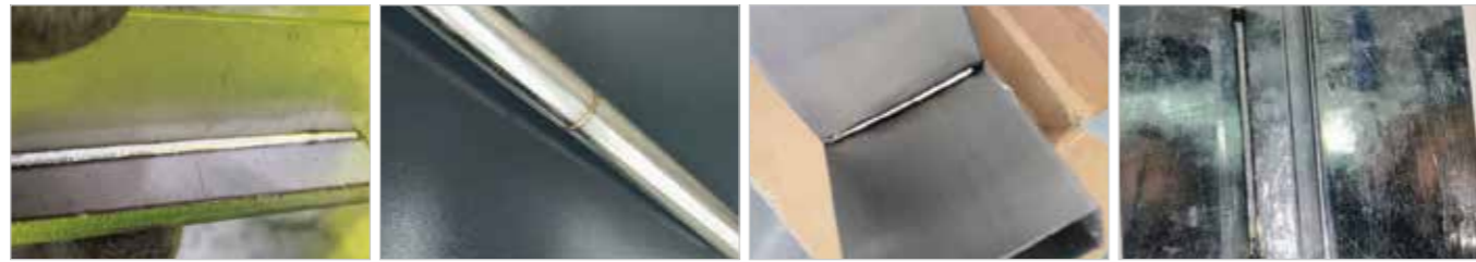
Stainless steel fillet welding
