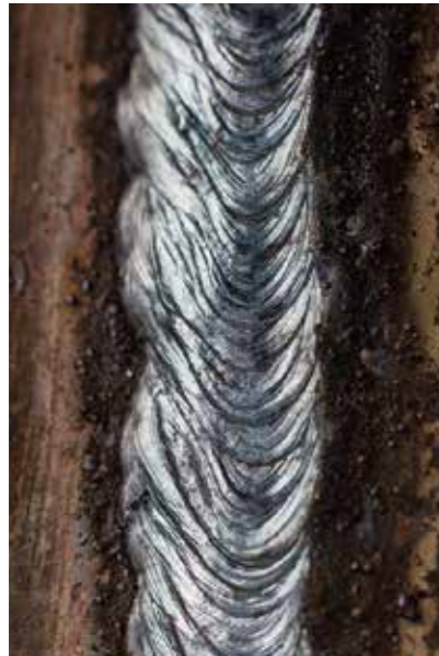
Unightly welding and high damage rate
